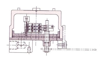
ULA - 003 EX, is exclusively designed for use in potentially explosive and highly inflammable atmosphere. It employs a "CAM", shaft and lever assembly to transfer angular input / linear travel into an electrically make/break arrangement for position feedback at any specific point of the total stroke / travel. The O-Ring sealing in the body and on the shaft gives total sealing against dust and moisture entry.
